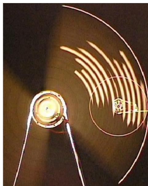
figure B.2 Experiment with two propellers, which swept areas are marked by the tracks of tip reflectors. The small propeller forces a stream through the swept area of the larger one, which has stall flags installed every 0.05R at its trailing edge. It can be seen that the flow separates and rapidly reattaches.
