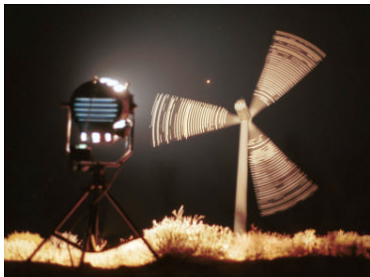
figure 3.1 Application of the stall flag method to the NEG Micon 700/44m at Tehachapi, Ca. USA.
